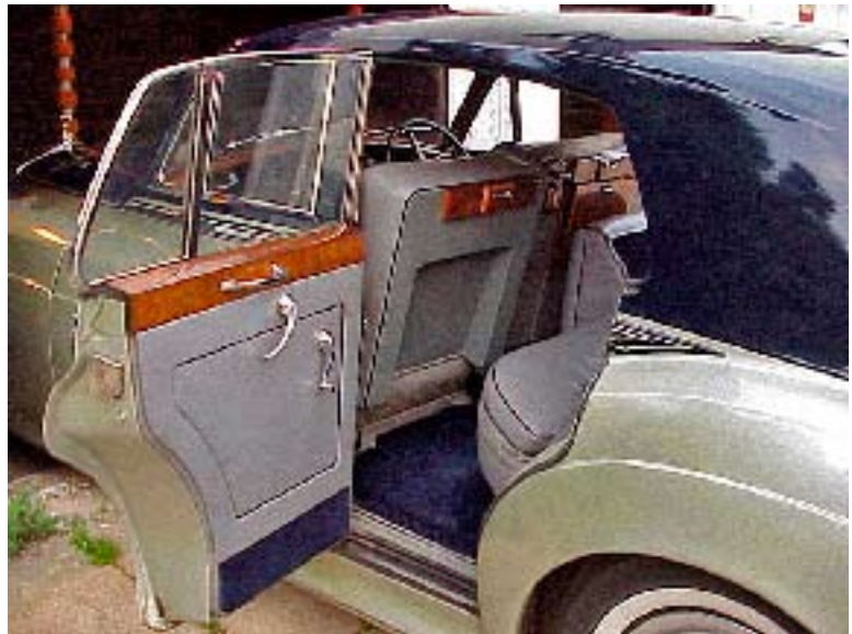
Front seat cut-out to provide more leg room for the rear passenger.
