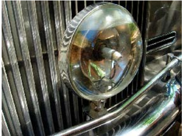
Rotofair light mounted to the front of the car can be pointed from side to side from the dash, like the current rave on the BMWs.
