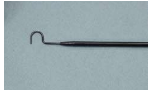
Figure 12 This blunt hook helped with installing the new seal / boot.
