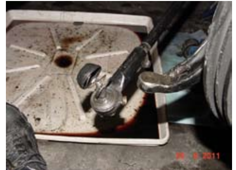
Figure 4 Ball Joint removed from the Side Steering Lever
