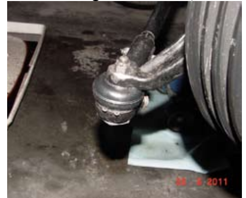
Figure 13 Rebuilt Ball Joint installed and ready for lubrication and service
