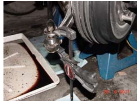
Figure 3 Using clamp to compress fitting, permitting removal of the castle nut.
