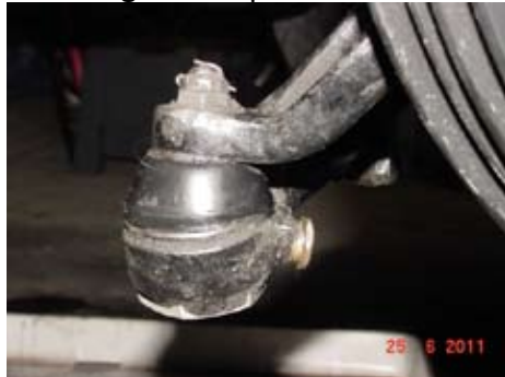
Figure 1 Old Ball Joint, grease coming out under the boot
